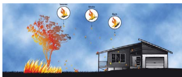
Embers ignite dry leaf litter in roof gutters
